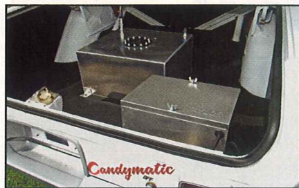
The thoroughly modern trunk of the replica Super Stock boasts a fuel cell and an aluminum battery box.
