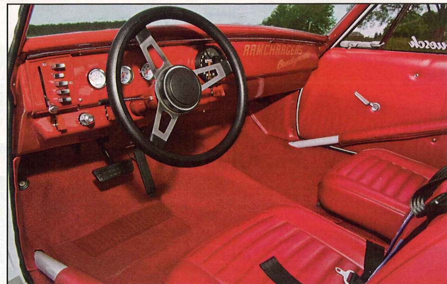
The interior of the tribute is not an exact copy of the original but rather a stylized version. The A100 van bucket seats seen here were used in the factory Super Stocks. Like the original, the tribute car has no back seat and is upholstered in red. Other factory Super Stocks we've seen had black carpeting, but the red-on-red color scheme is more attractive. The dashboard layout and steering wheel are a departure from the original. The button shifter doesn't display the reversed pattern that we've seen on 1964 factory racers, and, obviously, the Tuff wheel didn't appear until 1970.
